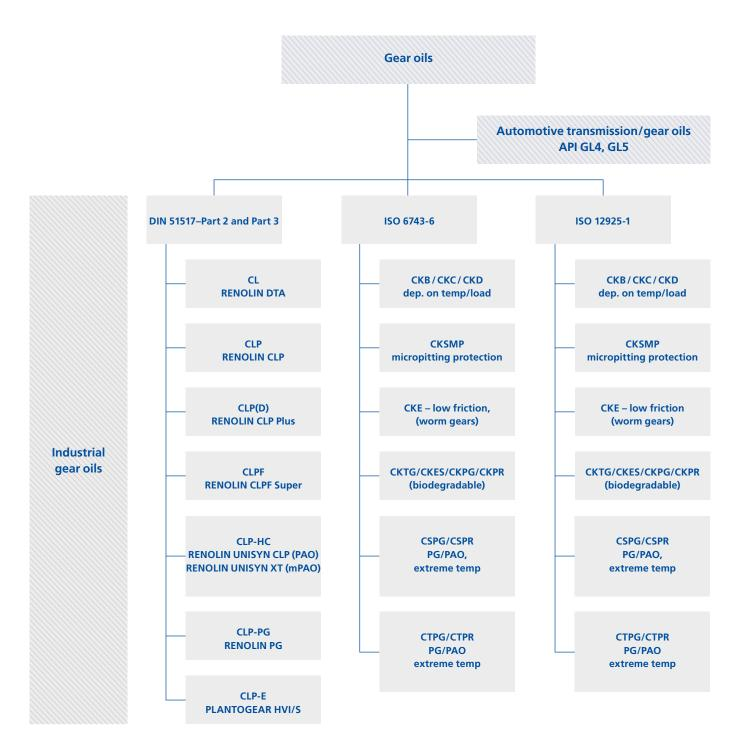
L = Anti-oxidants, corrosion protection (R&O)
