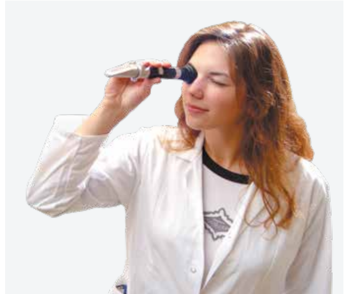
Fig. 2 – Correct use of a handheld refractometer
