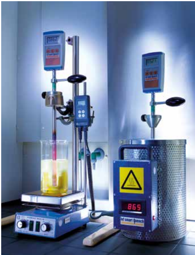
Fig. 6 – Apparatus to measure cooling time
