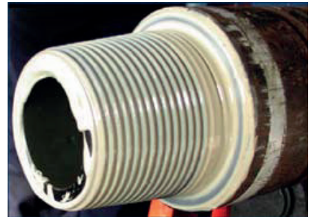
Figure 4 Drill pipe after first break-out
