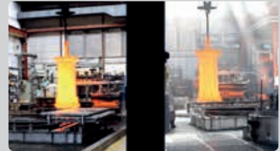
Comparison of flaming behaviour – universal high-performance quenching oil THERMISOL QH 35 MC (right in the video)
