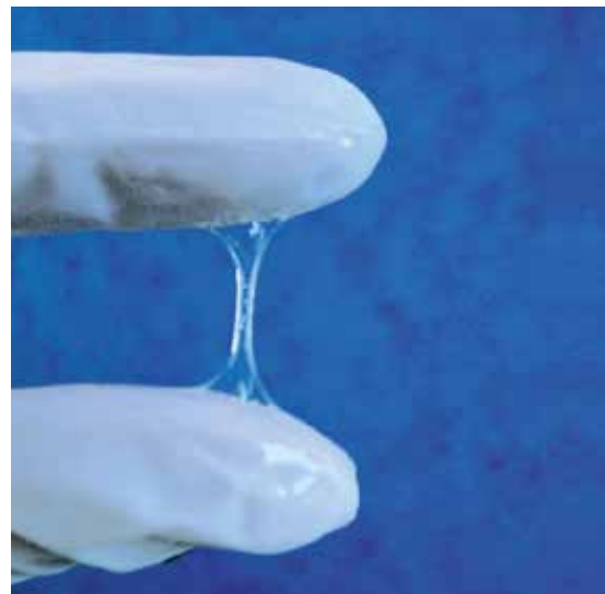
Slideway oil with "tackifier"
