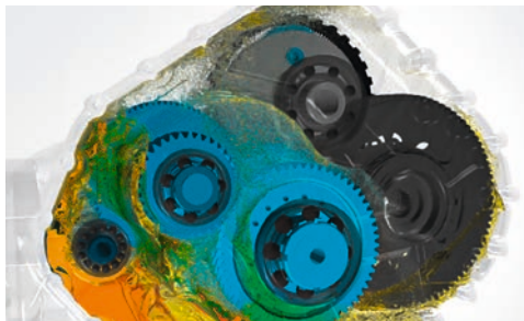
Simulation of the fluid flow in the high-speed transmission © FZG TU München
